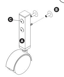
Loosely pre-attach sombrero nut (B) to screw (C). Do not tighten all the way.
