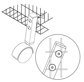
2 Insert rim of sombrero nuts through wire opening by first positioning caster leg at an angle, then turning straight as shown in next step.
