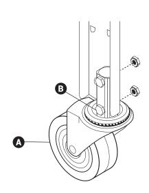
Caster kit attaches to leg supports for added mobility of cages.
