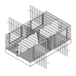
9 Using spring hook, attach cage to secure the tray during transport.
