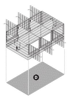
6 Attach flooring (D) to cage, two inch up from the bottom of side panels using cage clips every two inches.
