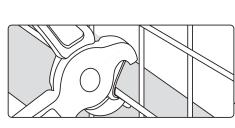
Insert pre-assembled partitions into cage and secure using clips at every slot.
