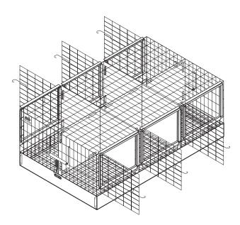
8 Using spring hook, attach cage to secure the tray during transport.
