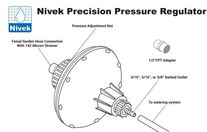
The Nivek Deluxe Pressure Regulator is an in-line device for reducing household water pressure to the low pressure required for an automatic watering system. It is a high capacity unit with a large diaphragm for the most accurate low-pressure regulation. The Nivek Deluxe Pressure Regulator is constructed of durable plastic making it very resistant to corrosion. It is designed to handle up to 600 drinking valves.
