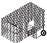
Snap door guards (C) around edges of door openings.
