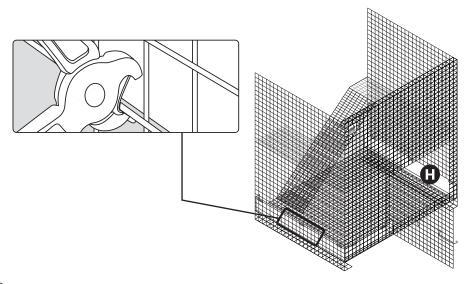
$oxed{3}$  Secure front and both side deflectors (H) to the cage using cage clips at each slot.
