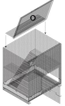
Attach top panel (D) to back edge of cage using cage clips.
