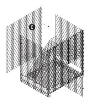
Attach back panel (C) to main panel assembly using cage clips every four inches where the panels meet. Secure back deflector now that back panel is secured to the cage.
